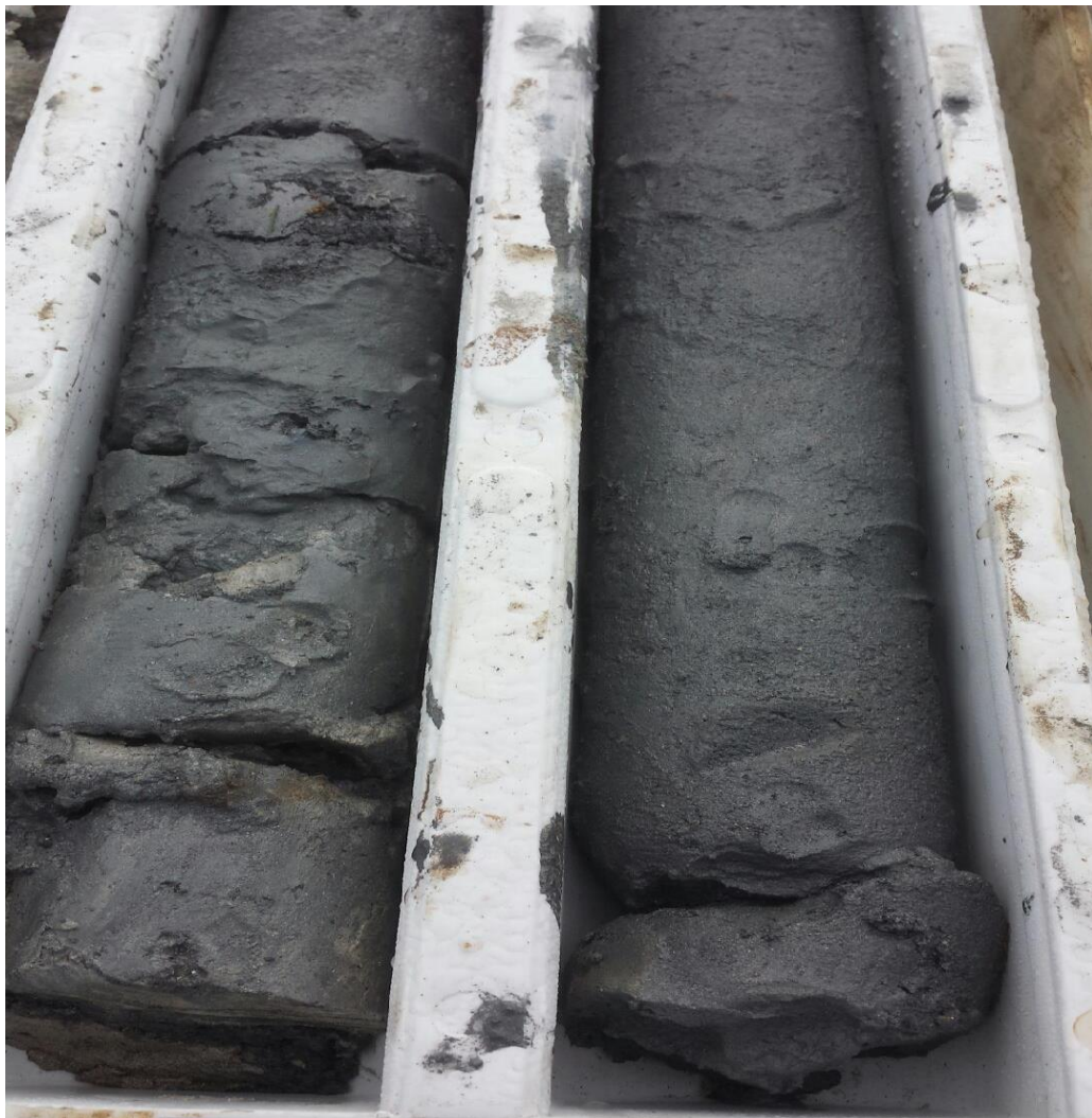
Close up of soft graphitic clays in diamond drill core
