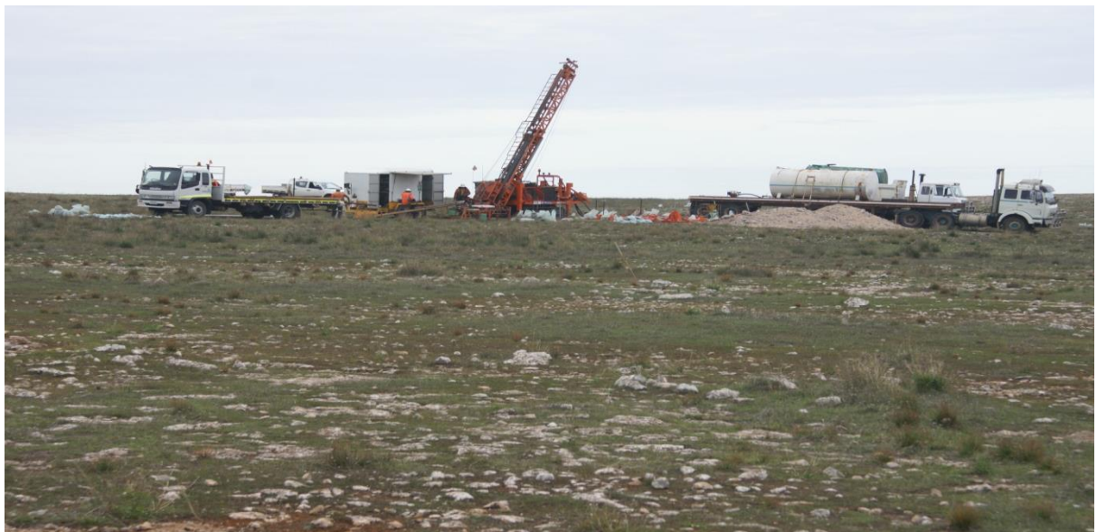
Diamond drilling to collect metallurgical samples for testing at Bureau Veritas in Adelaide
