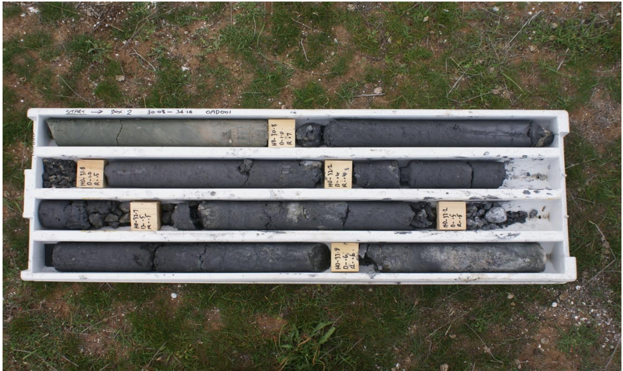
Soft graphitic clays interbedded with soft basic volcanic clays in diamond drill core
