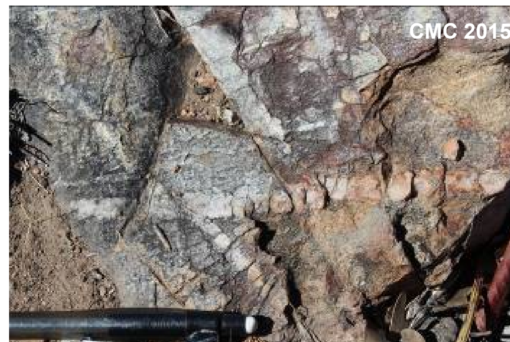
Quartz-Fe oxide bearing vein in silica-sericite altered rhyolite, Mt McLaren prospect.
