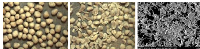
Figure 7: Proppant formulation 8602: Fired proppants (left), Crush residue (centre) and Scanning Electron Microscope image (right)
