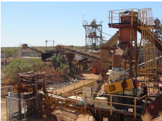
Crushing circuit including new secondary cone crusher and magnet, and Acacia Reactor installed in the upgraded gold room
