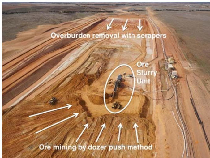
Figure 19: Strandline dozer push mining and processing
