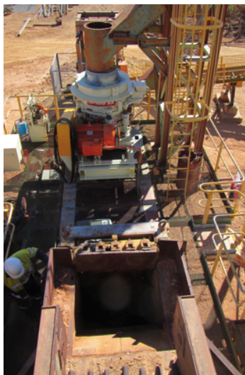
Crushing plant including new secondary cone crusher
