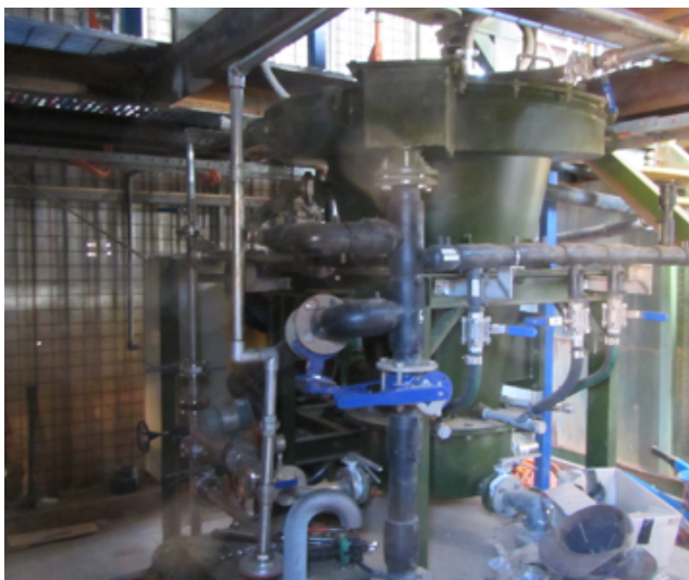
Acacia Reactor installed in the upgraded gold room, and the recently re-lined mill awaiting final works
