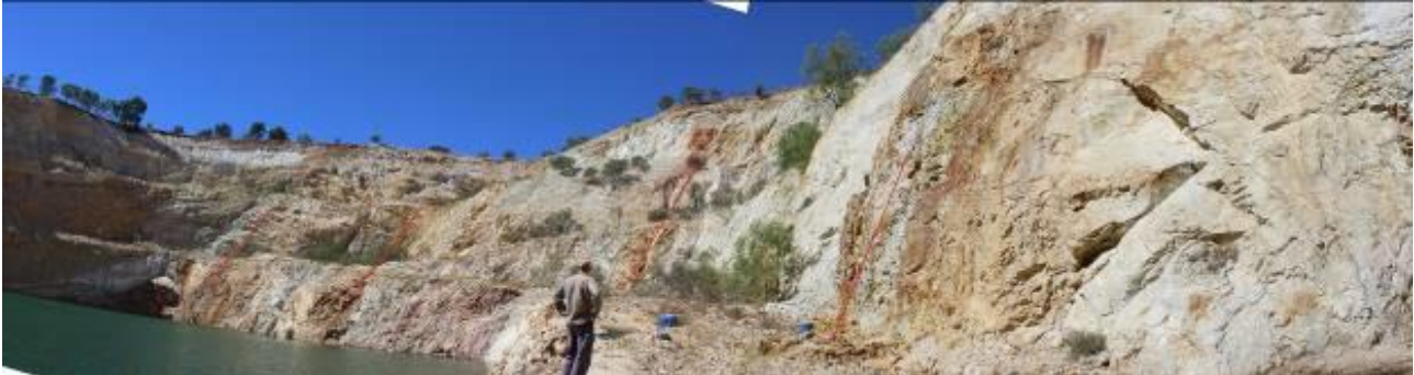
Figure 1. Quartz-pyrite lodes visible as sub-vertical, red-brown oxide zones in the Belyando pit wall (panoramic photo: D. Menzies, 2015)
