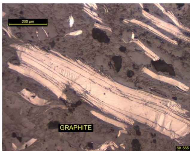
Figure 4: Sample SK555108 which assayed 7.25%TGC with 75% of the graphite flakes over 500 micron in length with 10% over 1,000 micron
