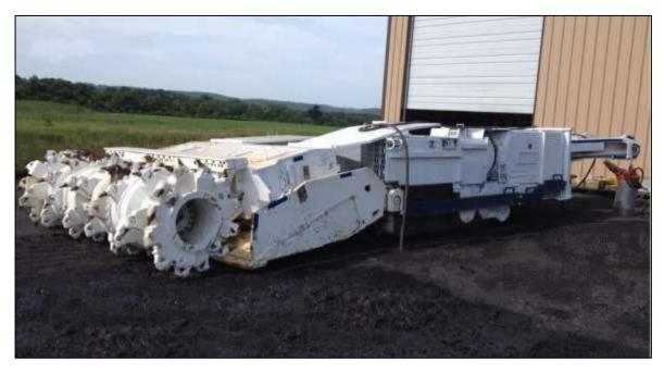
Figure 2 - New Continuous Miner Joy 14CM15 being commissioned on site at P8N
