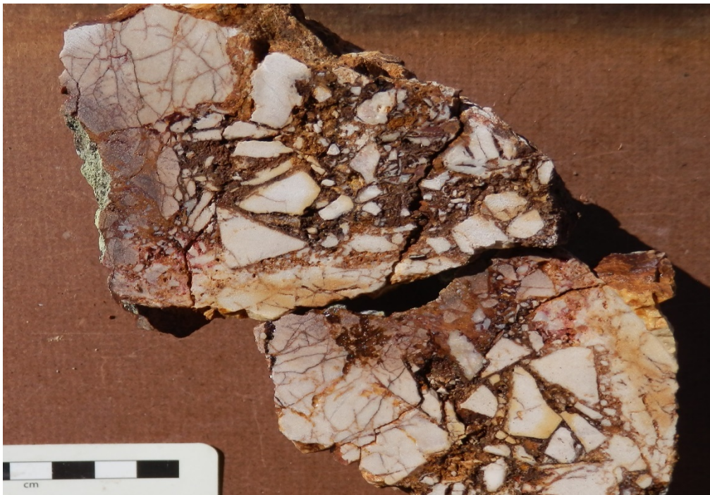
Figure 6. BAR016. Gossanous sandstone monomict breccia. 250 ppm As, 10ppb Au.
