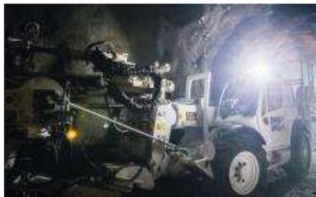
MDR700: Underground coring rig with advanced mobility and capable of wide drilling angles.
