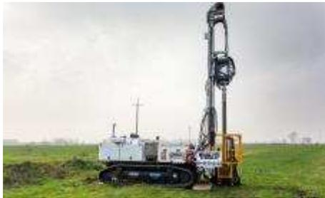
LS250 MiniSonic™ Rig: Compact footprint rig with a proven sonic head that delivers continuous 'in-situ' core samples.
