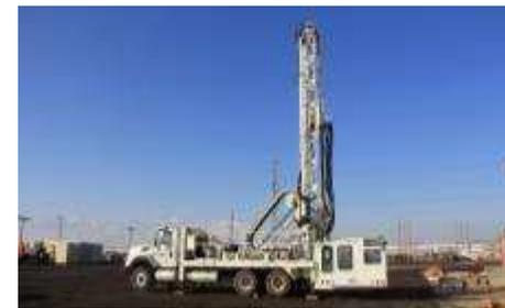
LF™350: Deep hole coring rig: 30 metric tons of pullback delivers high performance and productivity at significant depths.
