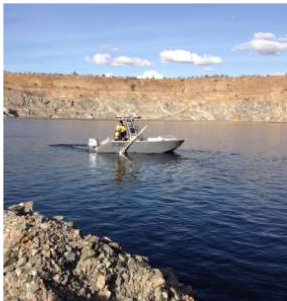
Figure 3: Eldridge pit (lower reservoir) Bathymetric Survey
