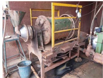
Primary grinding mill
