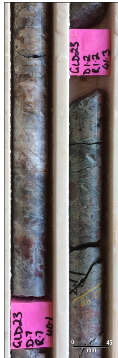
Photo 4: Hematite breccia at the interpreted Anna South vein position. GLD023 ~40m.
