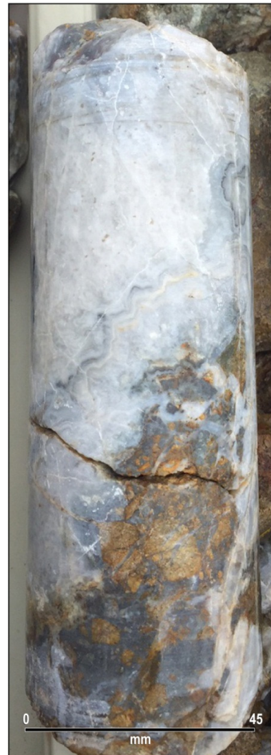
Photo 1: Quartz vein displaying colloform banding. GLD019 drillcore at 11.7 metres.
