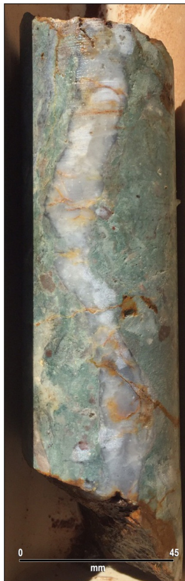
Photo 3: Pyrite rimmed quartz vein in brecciated rhyolite. GLD022 ~14m.
