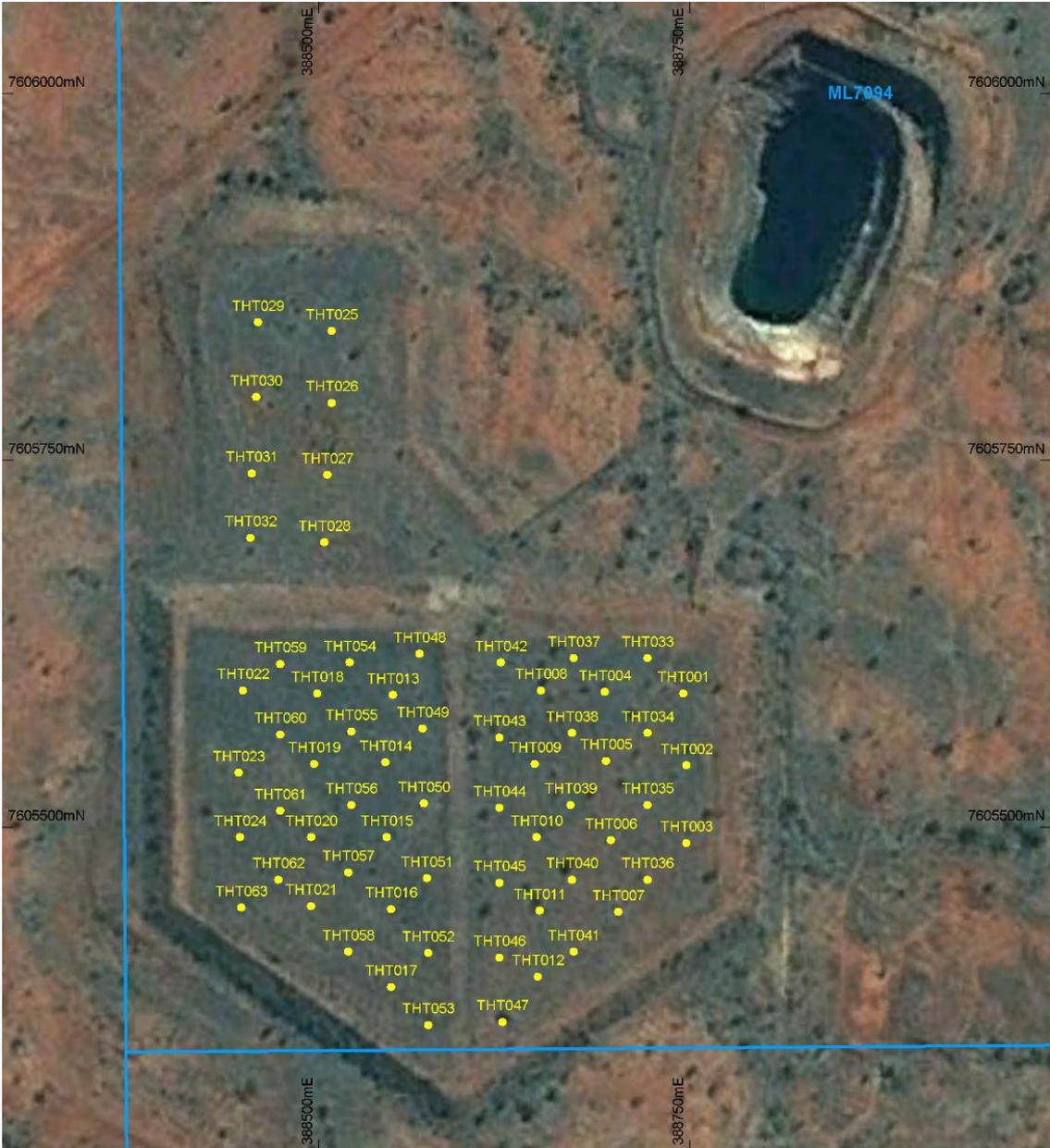
Figure 1. Tick Hill Tailings Storage Facility – First and Second Stage drill hole locations.
