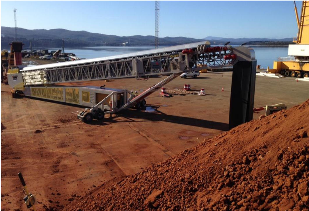
Radial stacker building bulk bauxite shipping stockpile at Bell Bay Port
