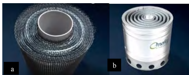
Picture #1 - a) rolled semi permeable membrane b) compact package
