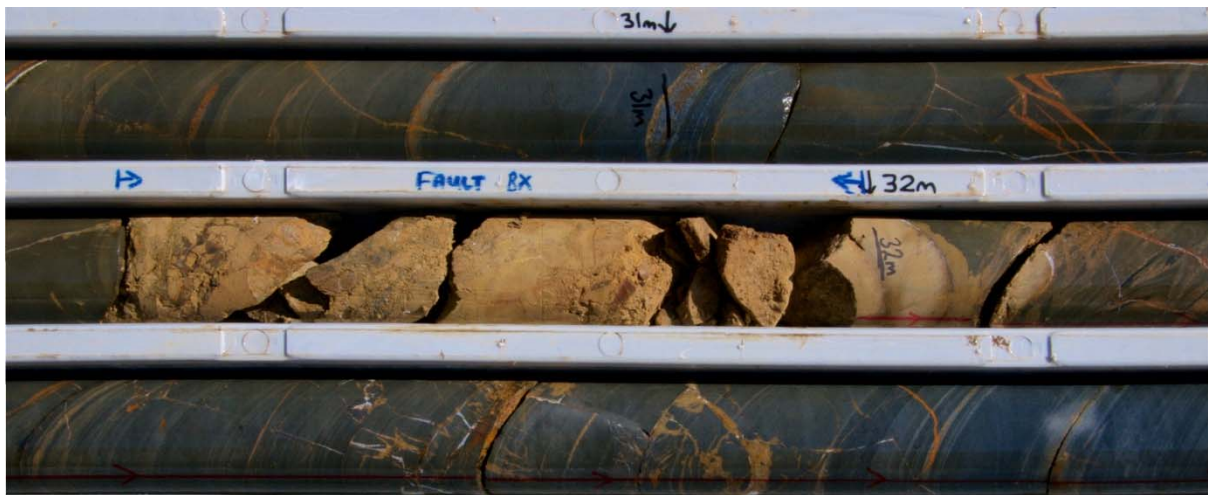
Figure 1. YRDH005 31.7-32m Oxidised fault breccia within laminated carbonate rich slate.
