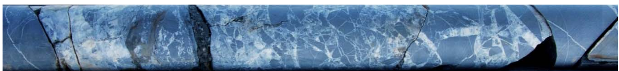
Figure 3. YRDH005 60.5-61m Brecciated slate with calcite/quartz matrix and black puggy (after sulphide).
