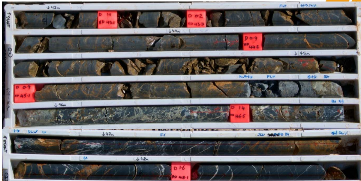
Figure 4. YRDDD005 44.2-48.1 Veining, faulting and brecciation within carbonate rich slate.
