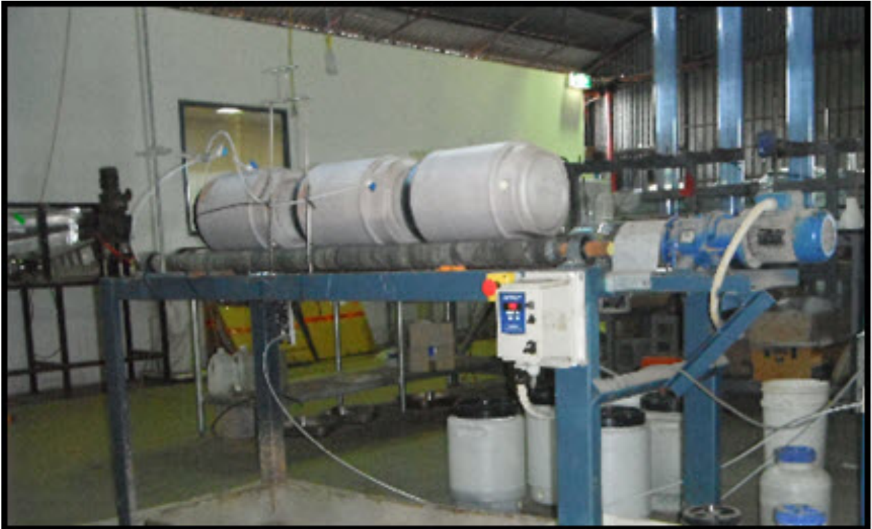
Figure 14: example of bottle-roll leach tests
