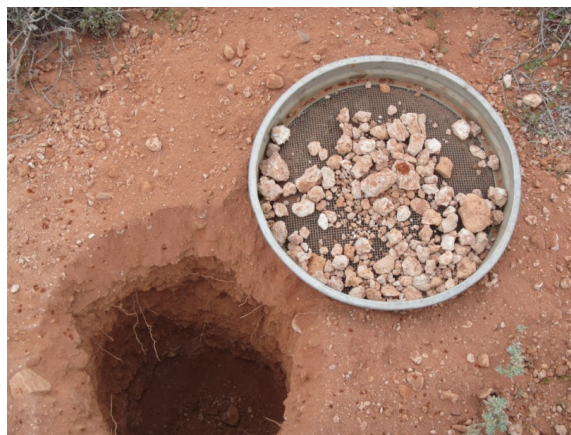
Figure 4: Typical calcrete encountered at the Widgety and Camel prospect included sheet calcrete.
