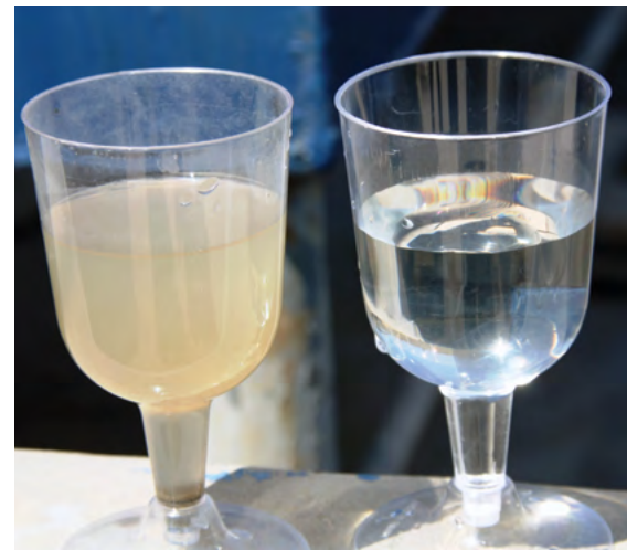
SABRE input and output water from demonstration plant.
