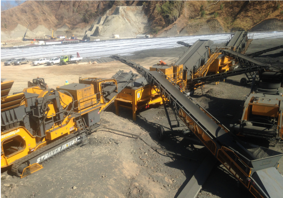
Image 2 – New crusher being commissioned on KKV leach pad
