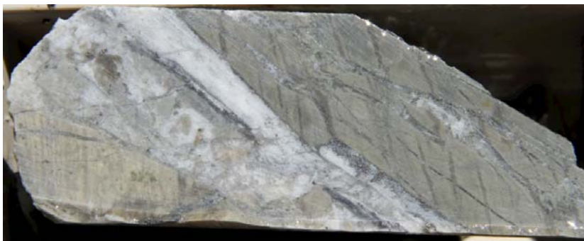
Hudson-McCrossins: Diamond drill core from hole HM-ZK0001, 63.1-63.25.m downhole. Altered metasediments exhibiting sheeted veining and brecciation infilled with quartz-carbonate-sulphide (NQ core, 47.6mm diameter)
