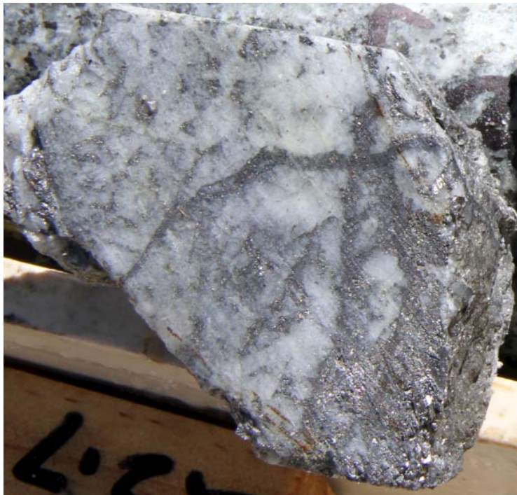
Frasers Find: Diamond drill core from hole FF-ZK0203, portion of sample H3, screen fire assay returned 2.17g/t Gold over 0.60 metres from 57.95-58.55m (Table 4). Quartz-sulphide vein (arsenopyrite, pyrite and lesser galena and sphalerite) emplaced within the Uralla Granodiorite (NQ core, 47.6mm diameter).
