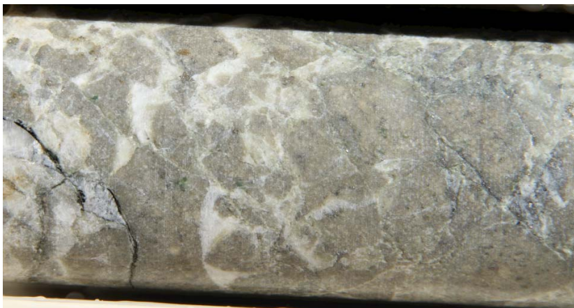
Hudson-McCrossins: Diamond drill core from hole HM-ZK0002, 37.40-37.50m downhole. Phyllic altered gold-bearing felsic dyke with disseminated sulphides (arsenopyrite and pyrite), quartz and carbonate flooded brecciation. (NQ core ,47.6mm diameter)
