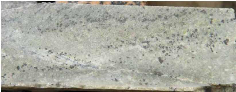
Hudson-McCrossins: Diamond drill core from hole HM-ZK0002 35.00-35.15m. Phyllic altered gold-bearing dyke that has undergone hydrothermal replacement by sericite, quartz, subordinate carbonate, disseminated pyrite and arsenopyrite. (NQ core, 47.6mm diameter)
