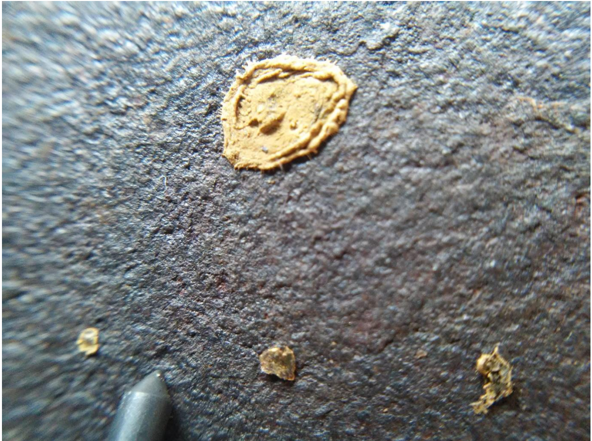
Fig. 1. Material resulting after amalgamation of saw cuttings and subsequent burning-off of mercury
