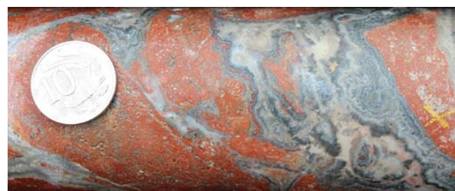
Figure 8: Drill core sample of colloform-textured epithermal quartz vein in sericite-hematite (brown areas) altered dacite (178.5m – hole MSDP05). Drill core width is approximately 6.4cm.
