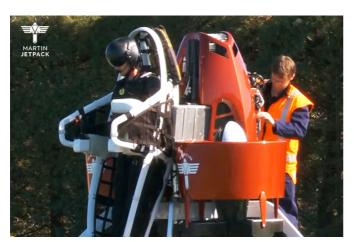
A new year and new beginnings as the Engineering team hands over to Flight Operations our next jetpack model for flight testing and evaluation. Designated P12.4, this new aircraft will join the jetpack fleet as a flight testing platform for both systems and component integration as we move forward to final design and production of the Next Generation Jetpacks (NG Model), which will be delivered to launch customers and partners later in the year.
