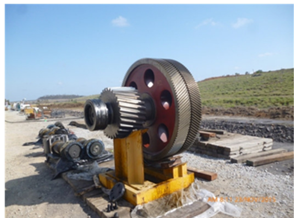
Drag/hoist input pinions
