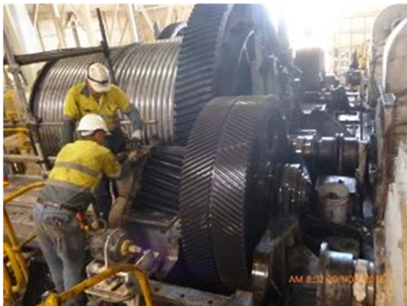
Removing hoist gearing
