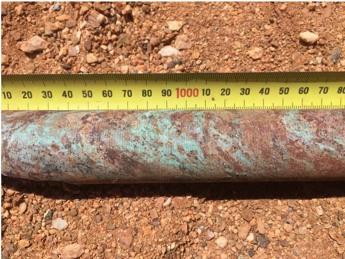
Figure 2 Mineralised core from hand held drilling at Rockface with pervasive malachite (copper)
