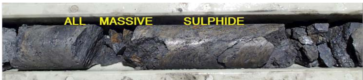
Interval 15.5 - 15.74m (100% core recovery): 31.7% Zn, 11.85% Pb, 0.9% Cu, 95g/t Ag - a massive sulphide lode (copper relatively low) - a width down hole of 0.24m
