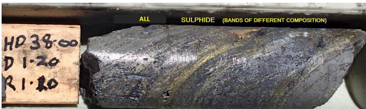
38.0 - 38.2m (approx) - all core is sulphide lode with very high average grade of 32.8% Zn - some bands with different composition are visible - banding to core angle 35 degrees
