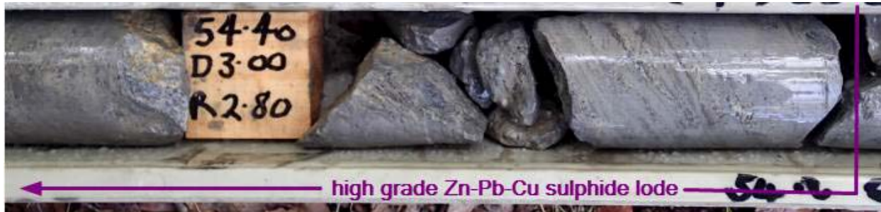
Interval 53.8 - 54.6m (0.8 metres downhole, 94% core recovery): 38.1% Zn, 8.0% Pb, 2.46% Cu, 60.7g/t Ag - a typical high grade zinc-lead-copper sulphide lode - note pale colour due to high zinc sulphide content and lack of pyrite
