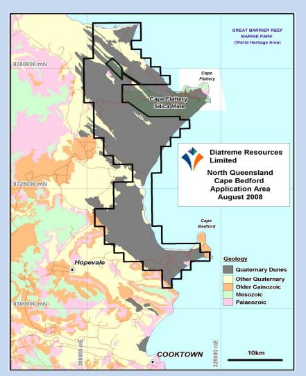
Large sand dune system with known silica sand and mineral sand occurrences over an area 50km x 15km in dunes up to 100m high.
