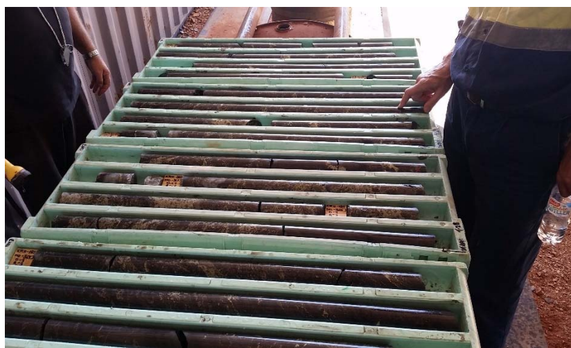
Figure 2. Core from drill hole KJCD183 at Rockface showing chalcopyrite in magnetite
