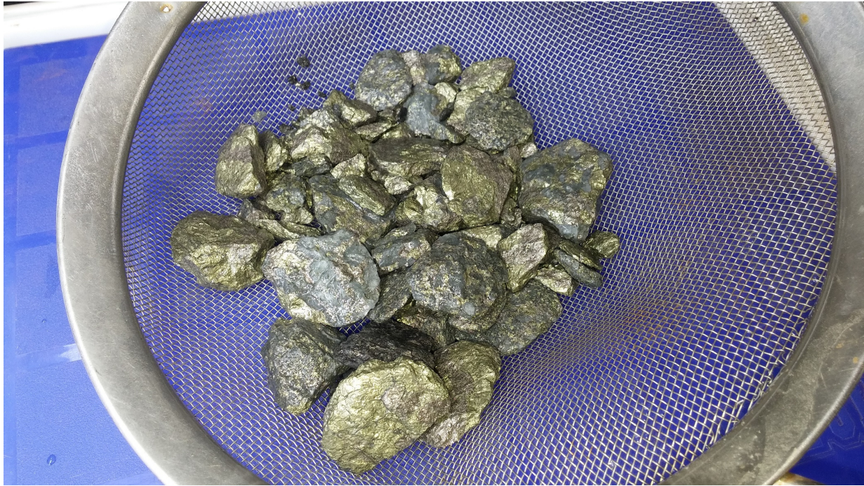
Figure 5 Sieved chips from drill hole AKC006 79-80m showing coarse chalcopyrite with pyrrhotite and pentlandite assaying 4.6% Cu 0.58% Ni 0.04% Co
