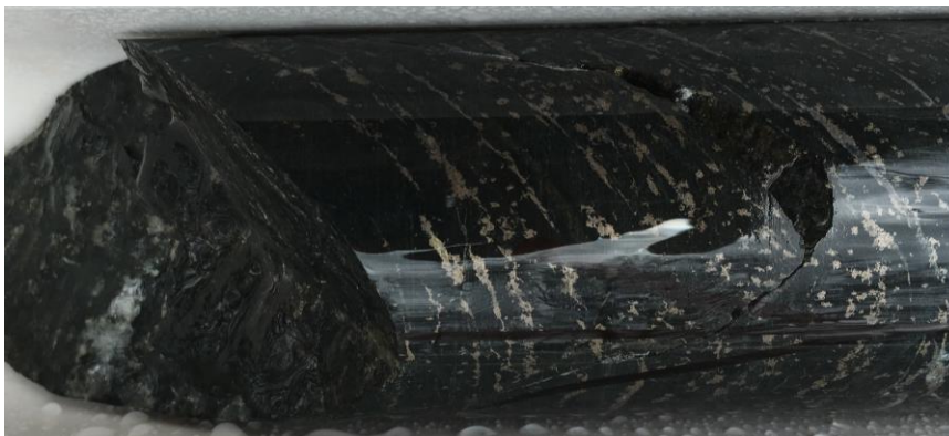
Figure 13. Syngenetic sulphides in TRBD013 at 412m downhole.
