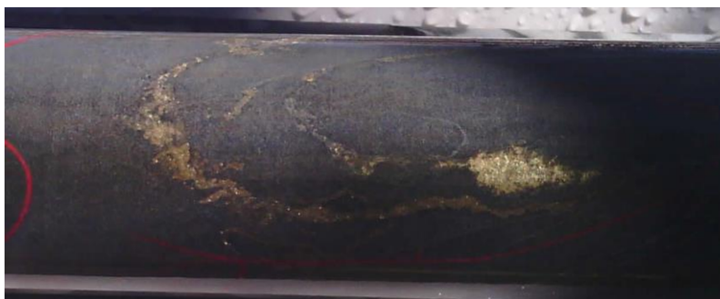
Figure 15: Remobilised chalcopyrite at 446m downhole in TRBD013.
