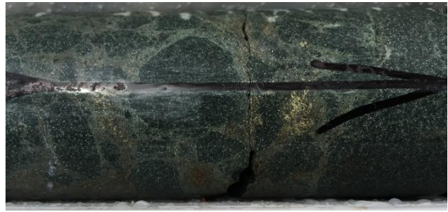
Figure 4. 399m in TRBDD013 at Impaler. Primary sulphide, possibly remobilised.
