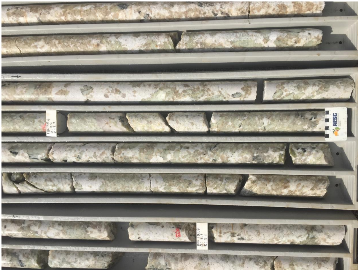
Figure 1. Large green spodumene crystals hosted by lighter coloured (white) feldspar and quartz. 95.2m – 103.1m FRDD001 (HQ), BP33 Prospect, Finniss Lithium Project NT.
