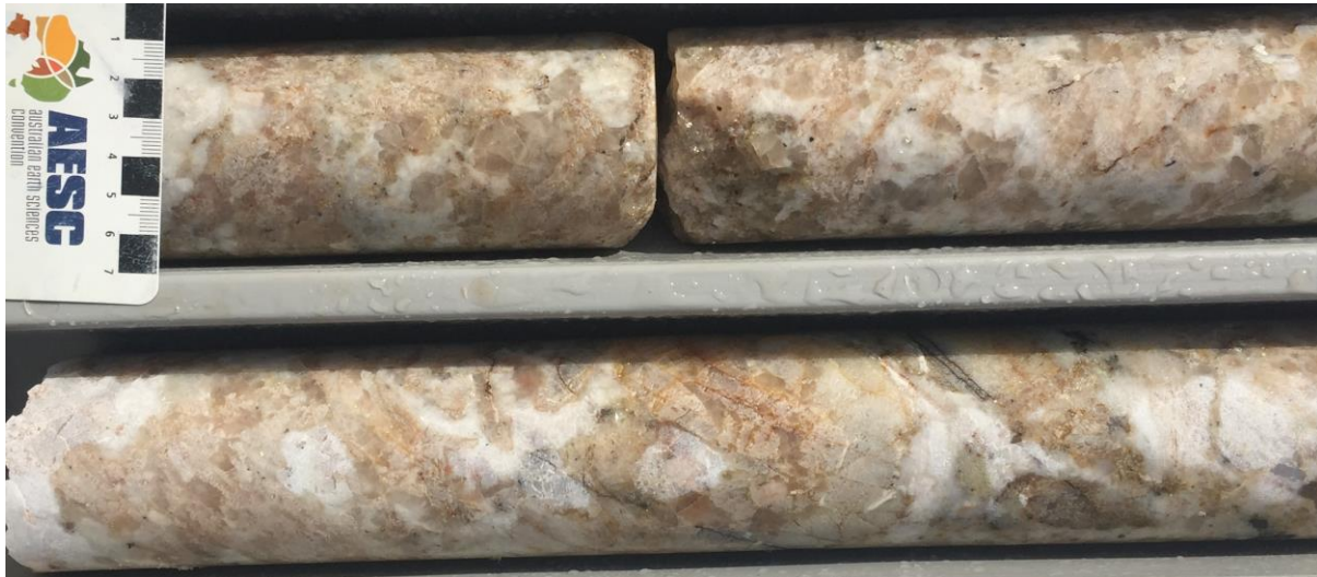
Figure 2. Pink/Beige spodumene making up a high proportion of pegmatite volume. 88.1m – 89.5m FRDD001 (HQ), BP33 Prospect, Finniss Lithium Project NT.
