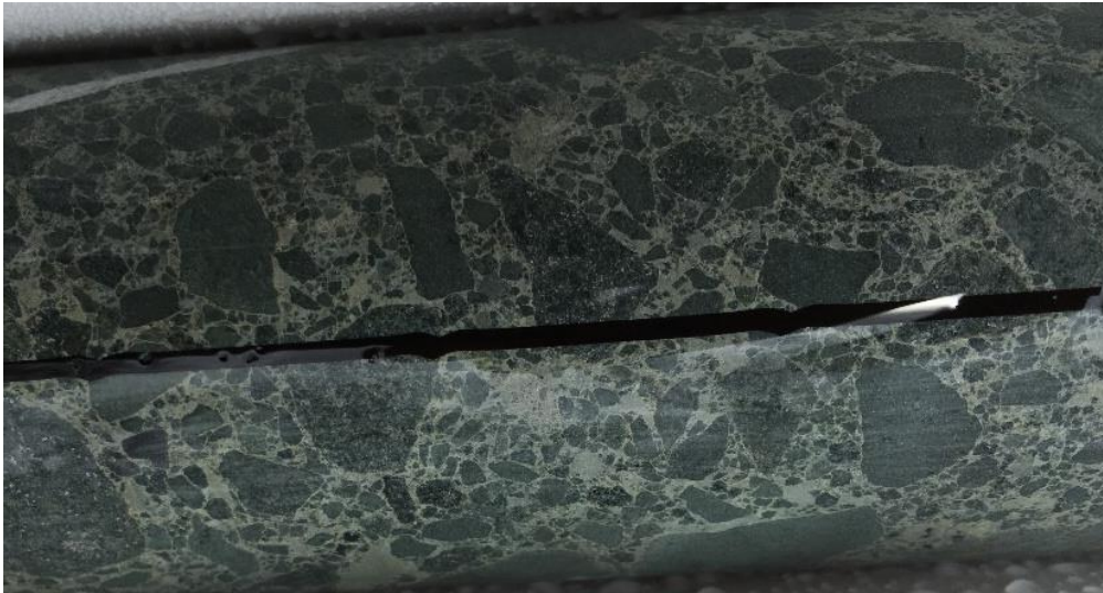
Figure 3. Peperitic texture: ~400m downhole in TRBDD013 at Impaler. Scale: core is 5cm wide.
