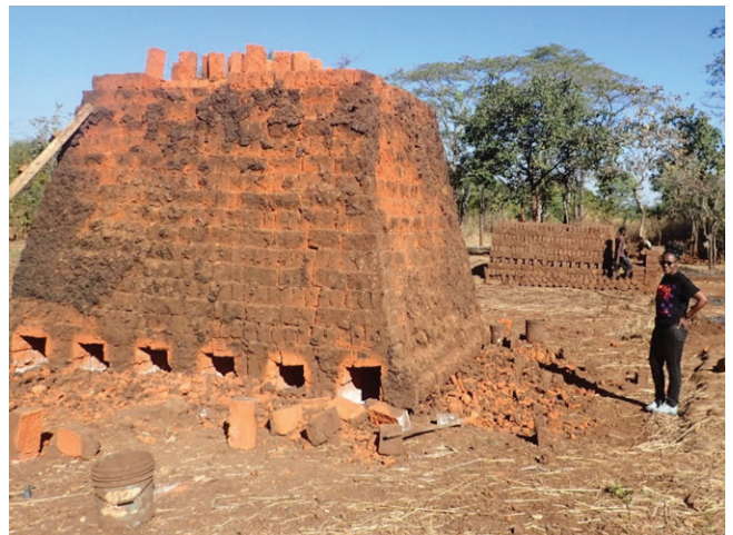
Figure 7: Brick kiln ready for firing for Magereza Primary School teachers houses project.
