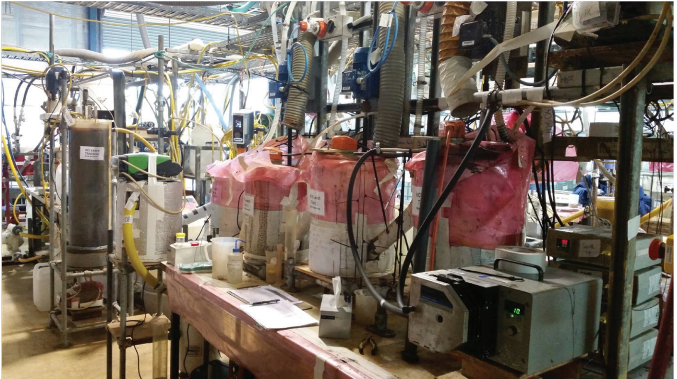
Figure 2: The acid leach section portion of the Leach Recovery Pilot Plant at ANSTO, showing the 4 leach tanks (mid-right) and thickener (left).
