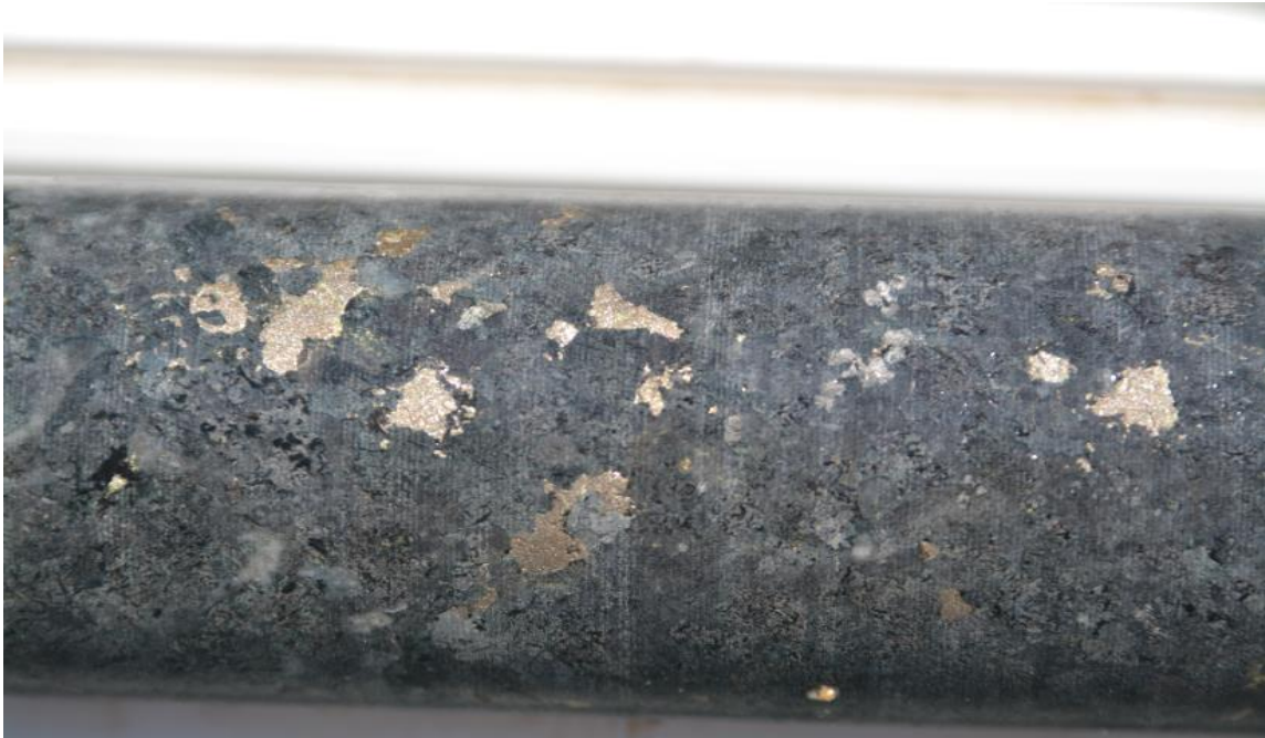
FIGURE 6: Globular magmatic nickel-copper sulphides (pyrrhotite-chalcopyrite-pentlandite) within coarse grained varitextured olivine gabbro at around 206 metres downhole in MRDD008.
