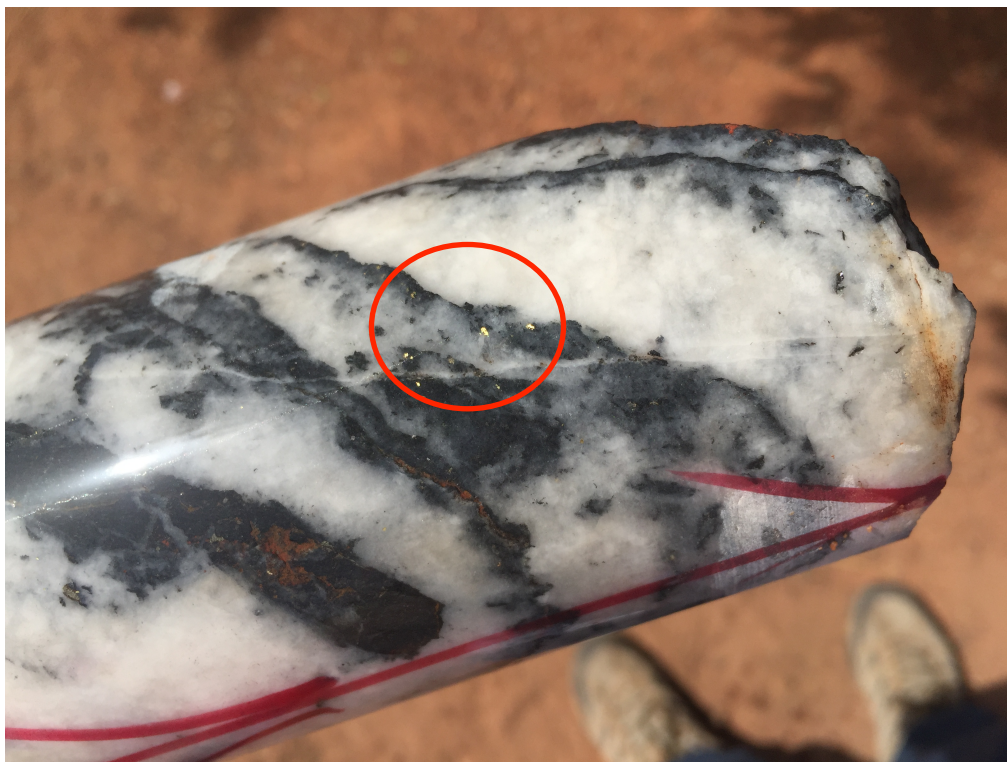
Figure 4: Drill core from DDDK16-002. Later stage quartz vein with visible gold (circled) and fragments of footwall graphitic sediments
