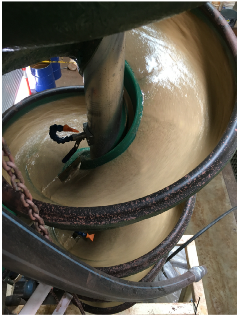
Image 1: Nolans 15 tonne bulk sample - commencement of gravity separation for the beneficiation pilot plant
