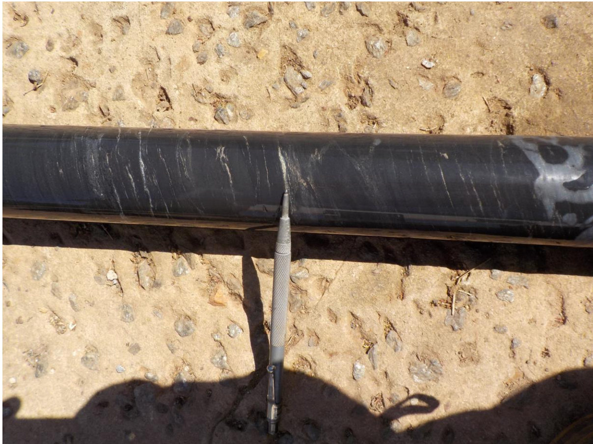
Drill core from PGPHD00182 (Mine Gate 1.), 147m depth: scribe pointing at a pyrrhotite - chalcopyrite lamina. Similar laminations are apparent in graphitic schist along the length of the core from 90m depth.
