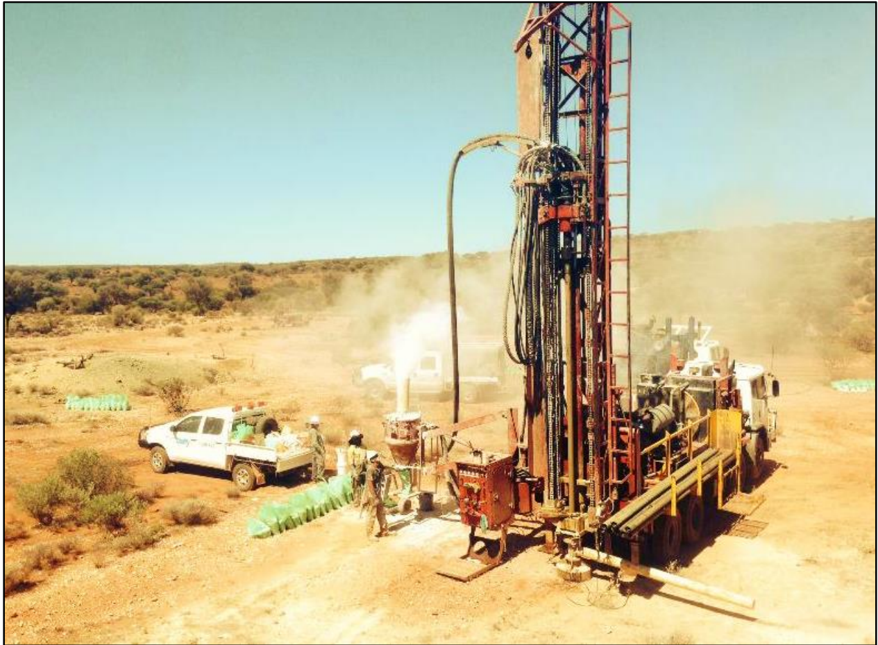
Figure 3: RC drill rig onsite at Torian's Mt Stirling Project.
