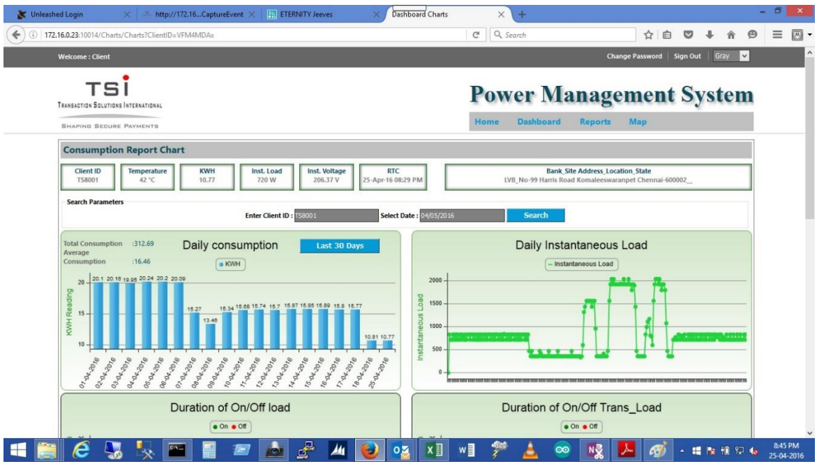
Image 4 – TSI India Power Management Control House tracking energy usage by appliance
