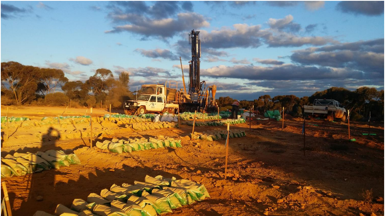
Figure 6: RC Grade Control Drilling at the Proposed Boorara Trial Pit Location.
