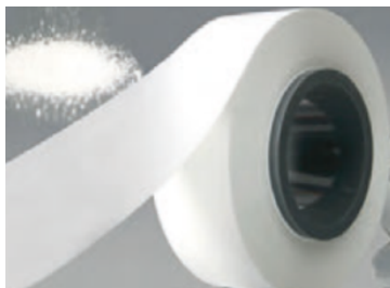
Figure 3. HPA-coated separator sheets on display at the CIBF
