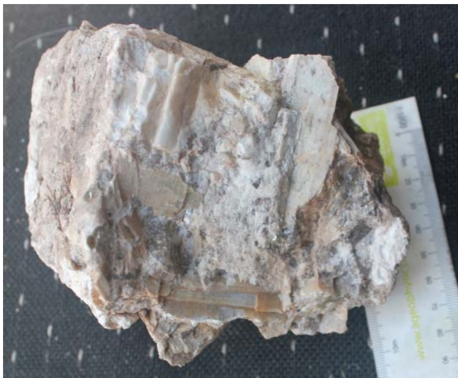
Sample 1123955: 1.81% \text{Li}_2\text{O} , from the Dempster L61 (L6100W) pegmatite. The large rectangular elongated minerals are Lithium-bearing Spodumenes.
