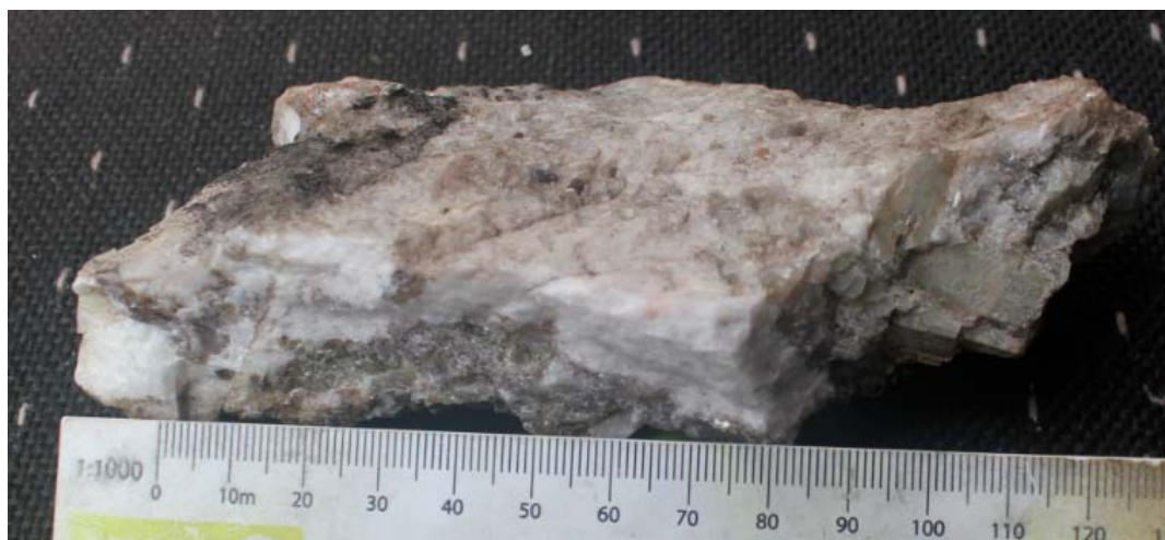
Sample 1123957, L2800W Sample 1123957: 1.08% \text{Li}_2\text{O} , from the Dempster L28 (L2800W) pegmatite. The large rectangular elongated minerals are Lithium-bearing Spodumenes.
