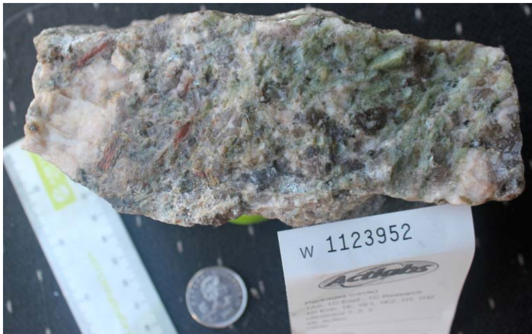
Sample 1123952: 0.55% \text{Li}_2\text{O} , from the Dempster L61 (L6100W) pegmatite. The large rectangular elongated minerals are Lithium-bearing Spodumenes.
