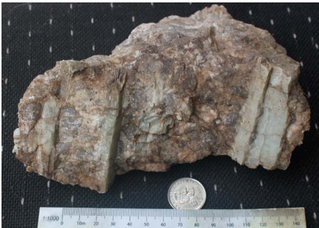
Sample 1123956: 1.84% \text{Li}_2\text{O} , from the Dempster L40 (L4000W) pegmatite. The large rectangular elongated minerals are Lithium-bearing Spodumenes.
