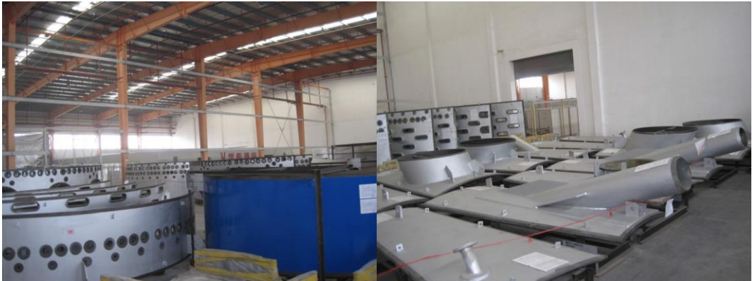
Blast furnace shell
