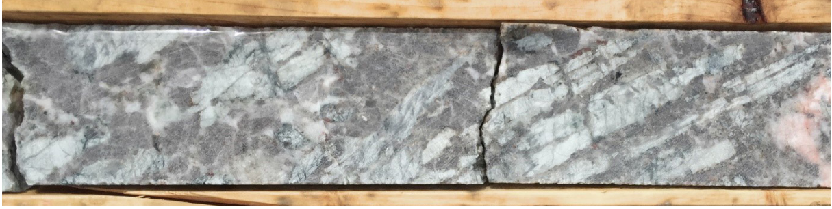
Plate 2: Intense spodumene mineralisation (white mineral oblique to core axis) in Falcon Lake West core.
