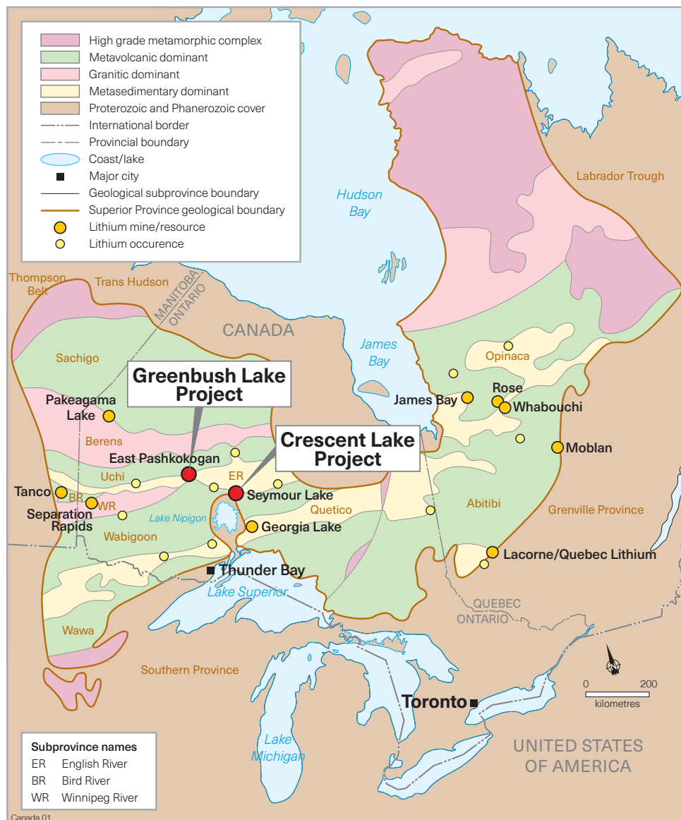
Figure 1: Geology of the Superior Province, Canada, showing Crescent Lake, Greenbush Lake and regional lithium occurrences.
