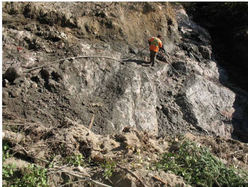
Figure 3. Worker washing down the newly excavated pegmatite structure located south of the North Aubry prospect to enable the geological team to review and identify the various lithium mineralisation zones.
