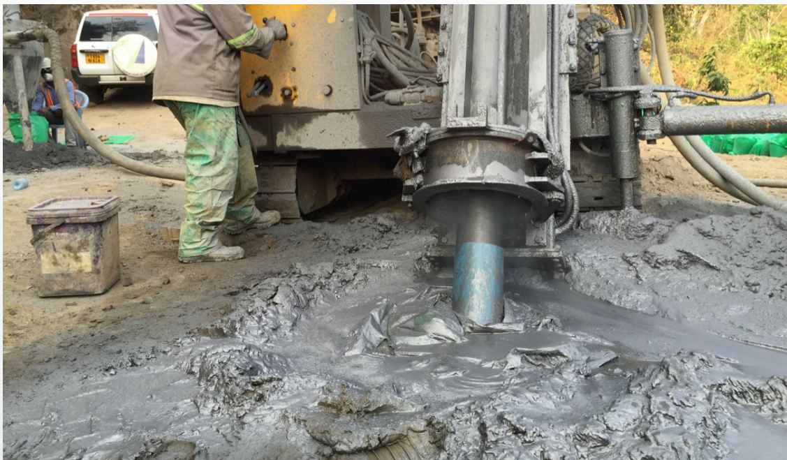
Photo 1. Drilling RC140 towards footwall at bottom of hole. Graphite being flushed out of hole with water. A diamond hole will be drilled along this line for metallurgical sampling and to compare RC Vs diamond drill method grades.
