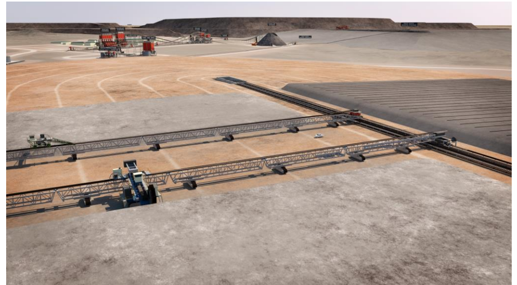
Proposed Etango Dynamic Heap Leach Approach
