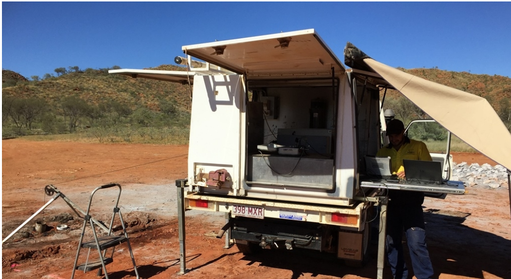
Figure 2 DHEM logging crew surveying KJCD199
